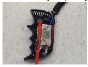
discovered that the inside consisted of two approximately two inch long resistors. The resistor on the left was connected to the live wires. The resistor on the right was connected to ground. The push-button has a shaft with a small metal piece attached. As the push button is held down, the metal piece slides down the resistors, making a connection between the two
